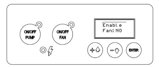
Use up/down buttons to switch to "Yes" and press "ENTER" to confirm. Turn off then restart pump for changes to take effect.
