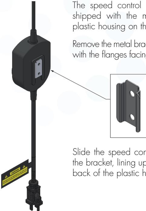
Slide the speed control housing down onto the top of the bracket, lining up the flanges with the grooves in the back of the plastic housing.
